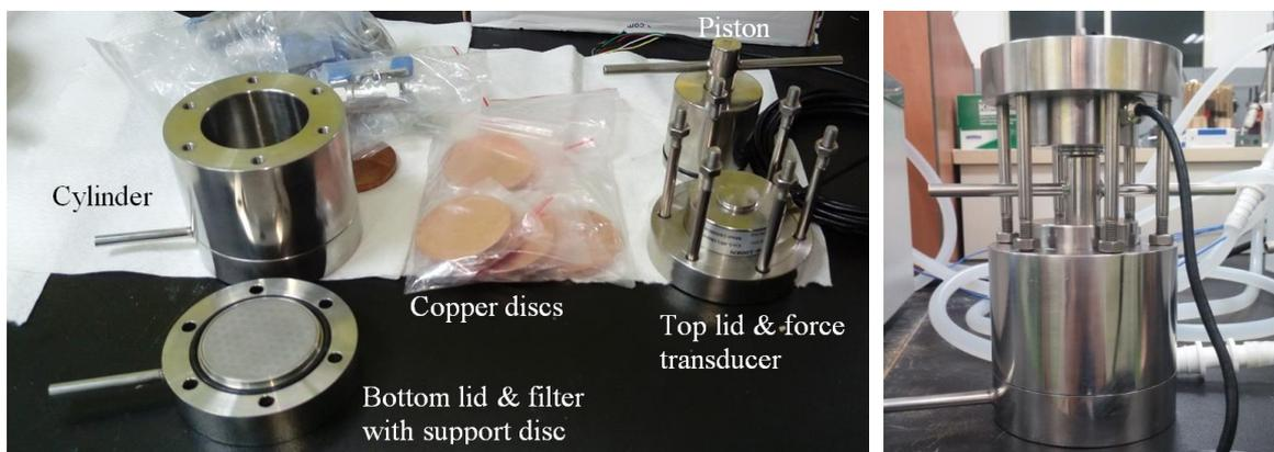
Figure 2-1 Left: Exploded view of the test cell. Right: Assembled form of the test cell.
